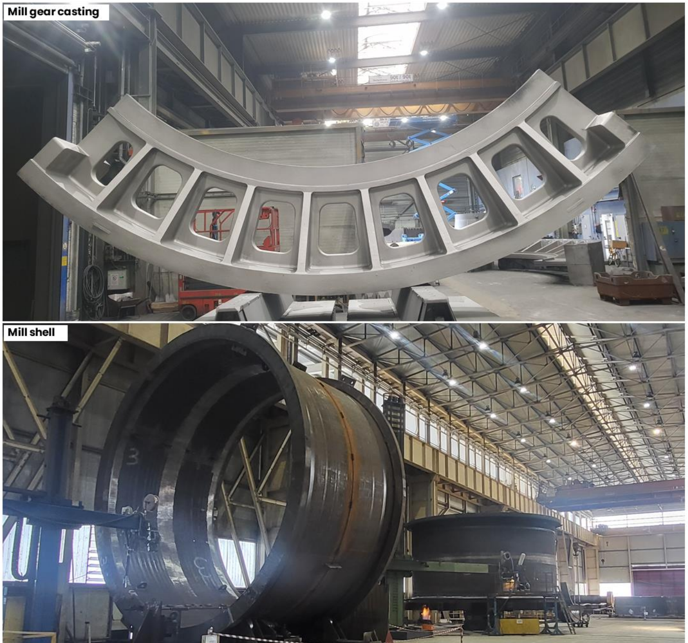
Figure 2: Mill gear casting and shell being fabricated
